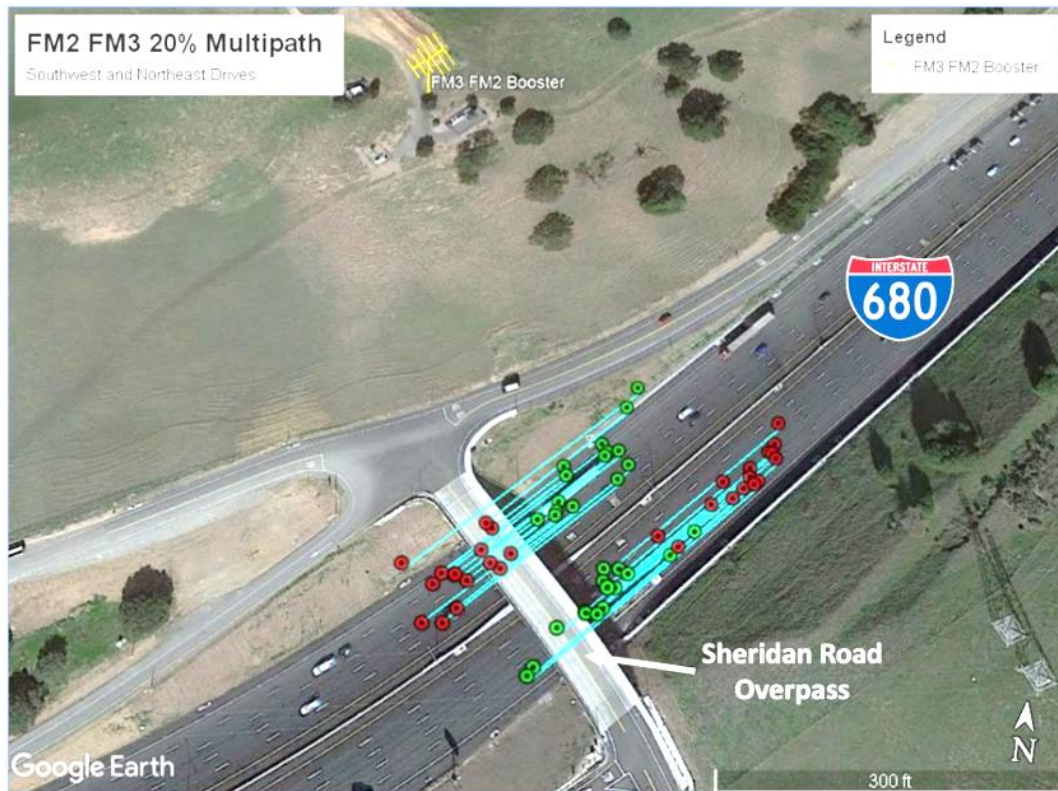
Figure 4 - Capture of Figure 12 used in Roberson KSJO report showing booster site and roadway where “Zone Transition Region” was measured.
