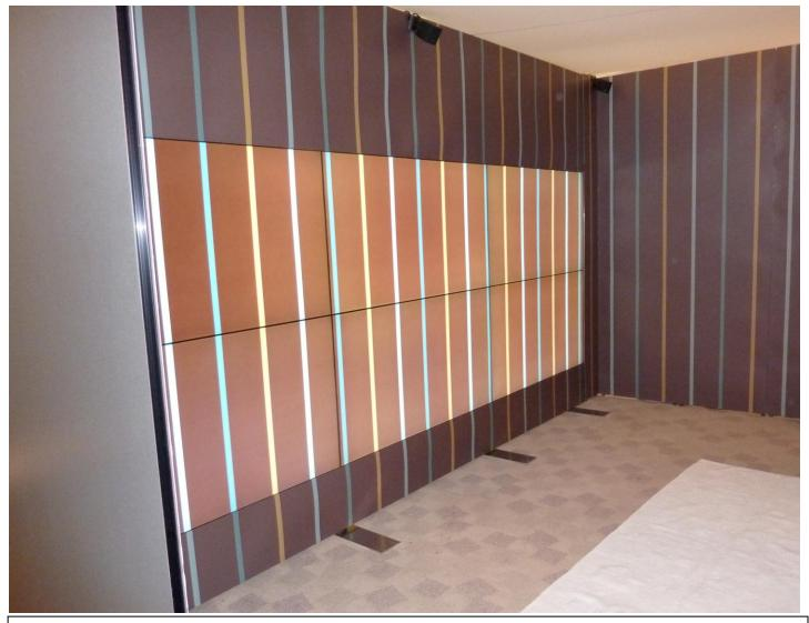
As demo participants entered the room, the default background of the screen carries through the wallpaper pattern. Without this feature, the blank display would present a large, dark rectangle that would likely be considered obtrusive to most consumers. For this demo, six 1080p LCD video-wall panels are countersunk into an opening in the wall, to simulate future ultra-thin displays that can be directly applied to walls.
