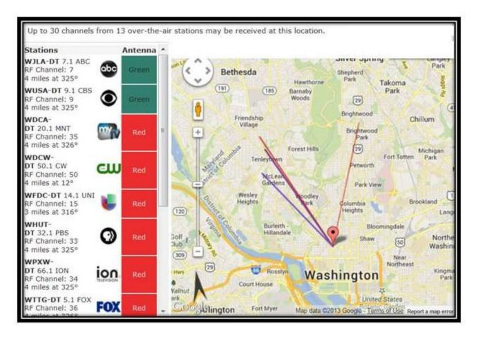
The map shows the direction and location of each local broadcast station and the color coding on the left identifies the type of outdoor antenna needed to access the various local stations. The antenna color coding corresponds to gain and directivity of antenna patterns according to the descriptions found under the Antenna Info tab on the app and at <u>antennaweb.org/Info/antennainfo</u>.
