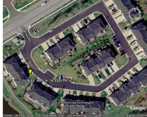
In this case, measurements were made immediately outside the townhouse to simulate the operation of a portable unlicensed personal device passing by the home. The signal level of station WFDC, DTV channel 15, was measured at the antenna location shown above and found to be at a level of -120.7 dBm. Accordingly, an unlicensed portable device with a sensing level of -114 dBm would conclude that the DTV channel was vacant.
