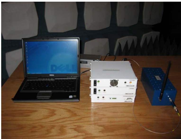
Figure 2-1. WSD Prototype A Sensing and Transmitting Device
