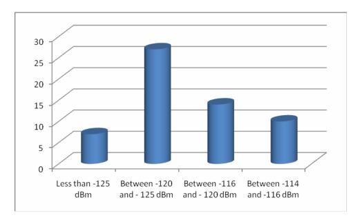
The above chart shows the distribution of measurements below -114 dBm. As can be seen from the above chart, seven measurements were at -125 dBm and below; 27 measurements were between -120 and -125 dBm; 14 measurements were between -116 and -120 dBm; and, ten measurements were between -114 and -116 dBm.
