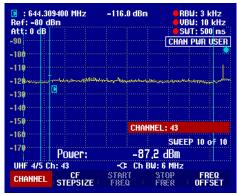
Both of these sets of measurements show locations and frequencies where spectrum sensing at levels below -114 dBm would result in harmful interference to nearby television reception.
