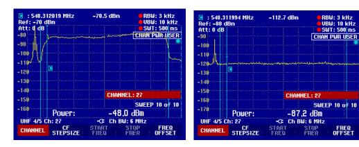
The above displays show the measured power of the pilot carrier on channel 27 at site 3 at both locations (Locations A and B). The pilot carrier power is displayed on the top center part of the spectrum analyzer display on the same line as the pilot carrier frequency.
