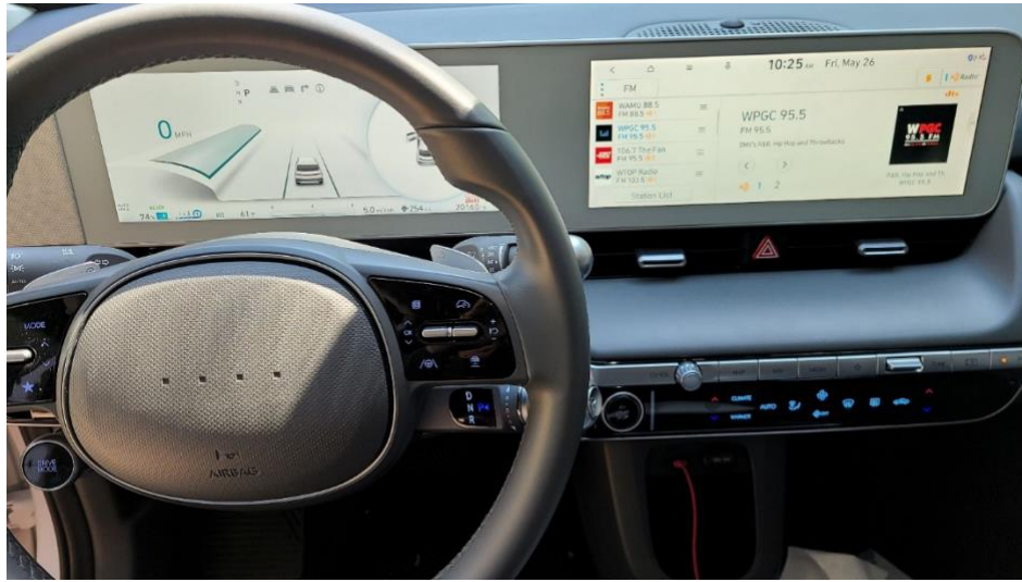
Dashboard of the 2022 Hyundai Ioniq 5 electric vehicle. Screen on the right is a touch screen used in conjunction with hardware buttons below to access vehicle functions.
