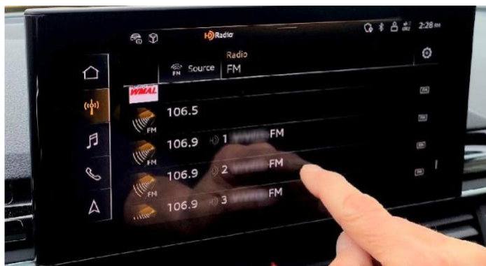
2021 Audi A4 hybrid radio showing FM band station guide with logos absent.
