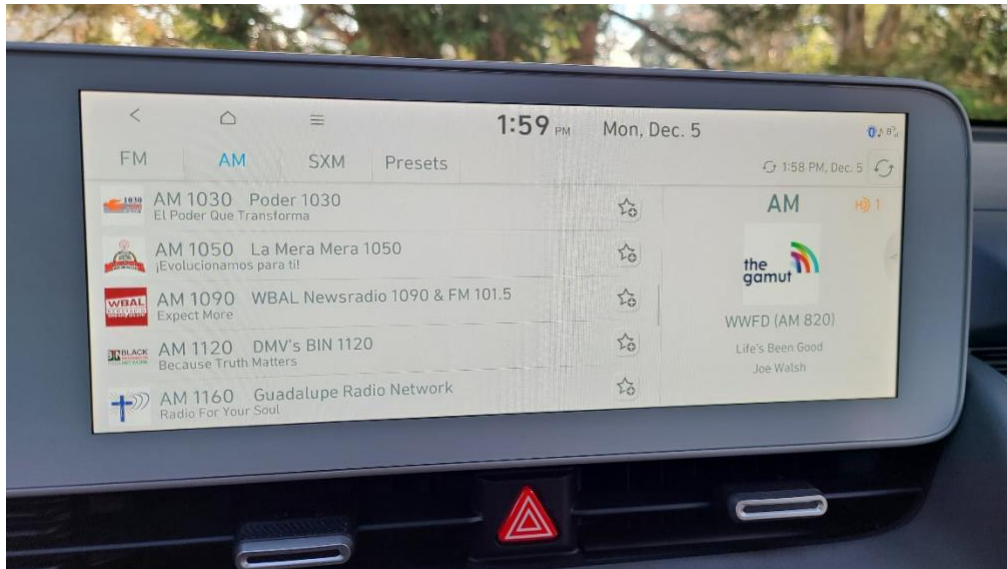
Ioniq 5 AM “Now Playing” screen using DTS AutoStage, with favorites list at left.
