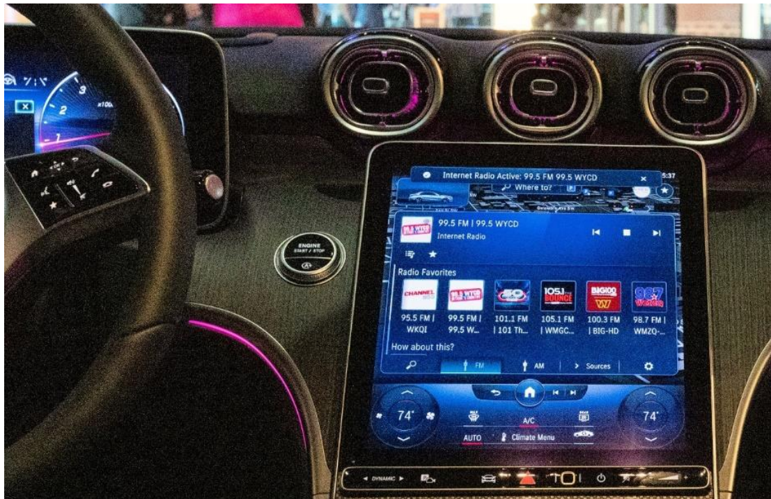
“Favorites” screen in the Mercedes C-300 sedan. These favorites can include a streaming version of stations that were at one time receivable over-the-air in the vehicle but are now out-of-market.
