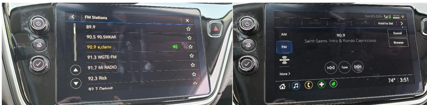
Chevy Bolt EV infotainment screen when displaying the FM radio station list (left) and a typical FM station “Now Playing” screen (right). As this is an RDS-only radio (no HD Radio), only text is displayed when the radio is in use.
